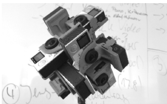
Fig. 3. Rig with mounted GoPros
