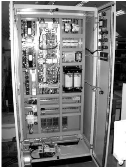
Fig.4. Power electronic conversion system ( P=30 \text{ kWt} ) worked out by "TWERD" Power Electronics Company
