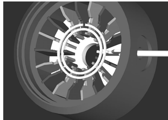
Fig. 5. Typical slow-wave structure
