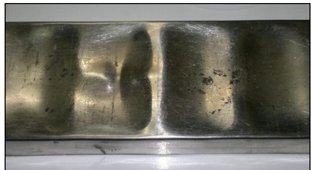
Fig. 9. Deformation of the working chamber EMD
